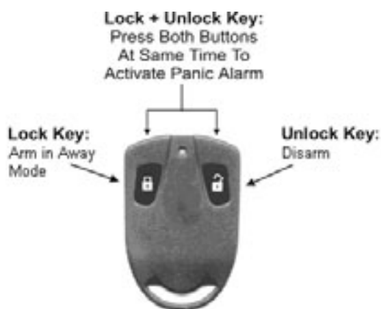
Figure 2: Two Button RF Keyfob (RF3332E)
